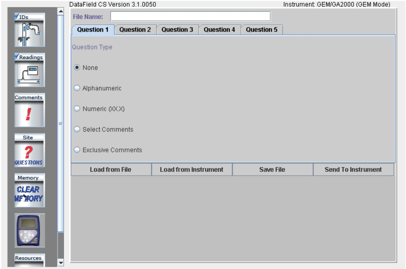
**Note:** Site questions must be created and sent to the instrument by the software prior to going into the field. They can not be hand inputted into the instrument in the field.
