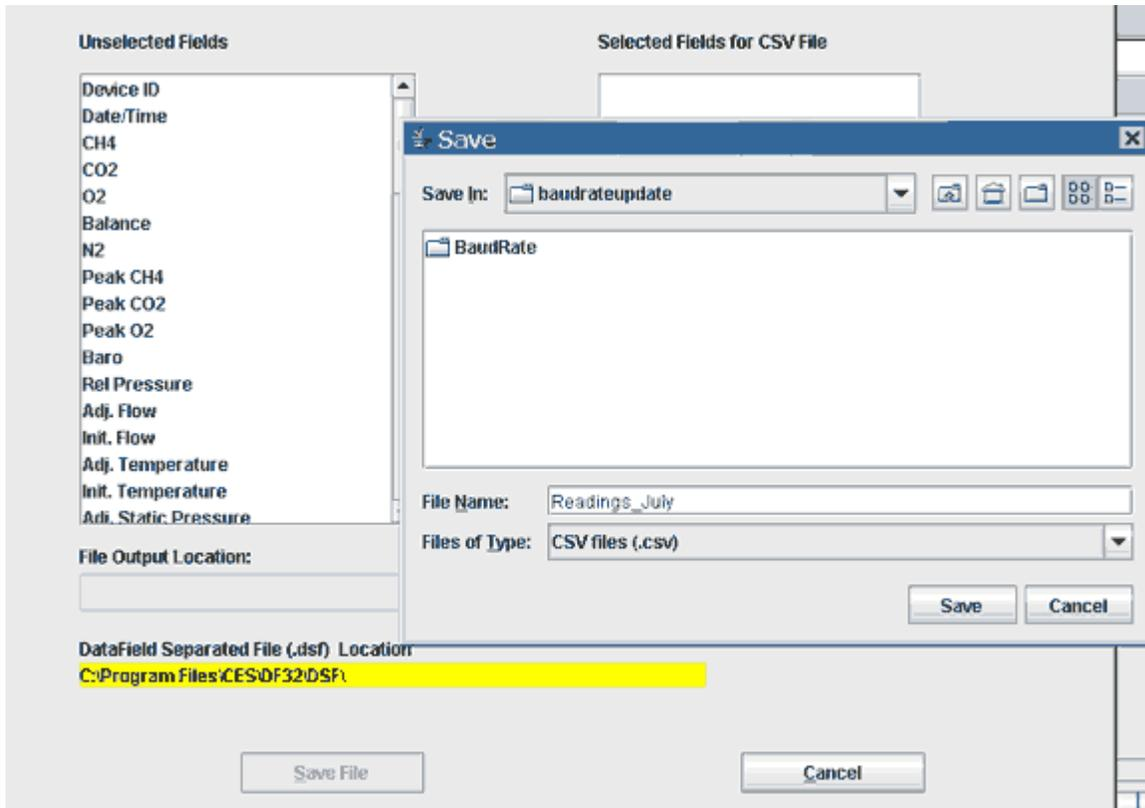
Note: If you load from file and you must be sure and load the dsf original file. The dsf files will all be save at the location you have set the path for
