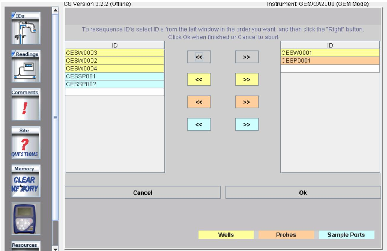
Select the ID from the left side window and click on the **Right** button to move ID to the right window to create the new sequence order. Repeat this process moving all IDs to the right side in the desired order.
