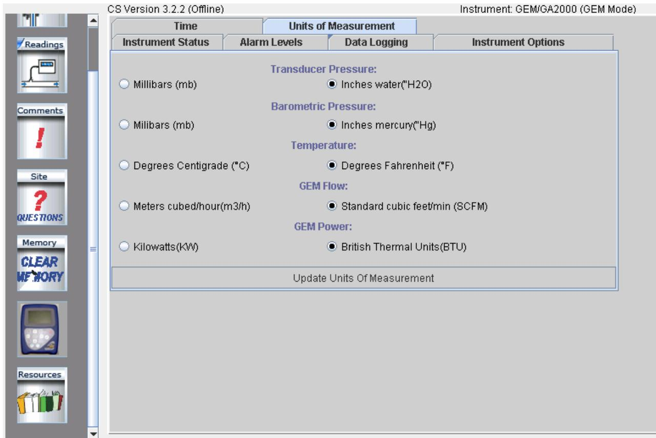
**Note:** EXTREME CAUTION should be taken if changing the Units of Measurement. All data from the instrument should be downloaded and stored in both, the GEM and the GA modes before updating the Units of Measurement. Updating Units of Measurement will erase readings from the instrument. The instrument should be turned off and restarted once the units of measurement have been updated.
