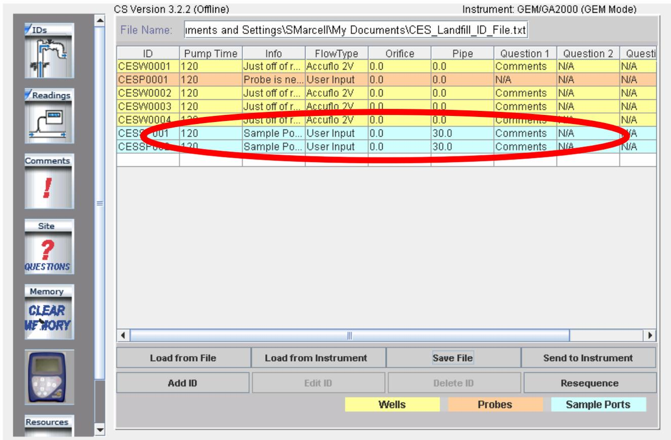
**Note:** It is suggested to clear ID information from the instrument prior to uploading the re-sequenced ID list. Otherwise the new ID list will be appended to the existing list. Clearing IDs in the instrument will clear IDs in the both GEM & GA modes of operation.
